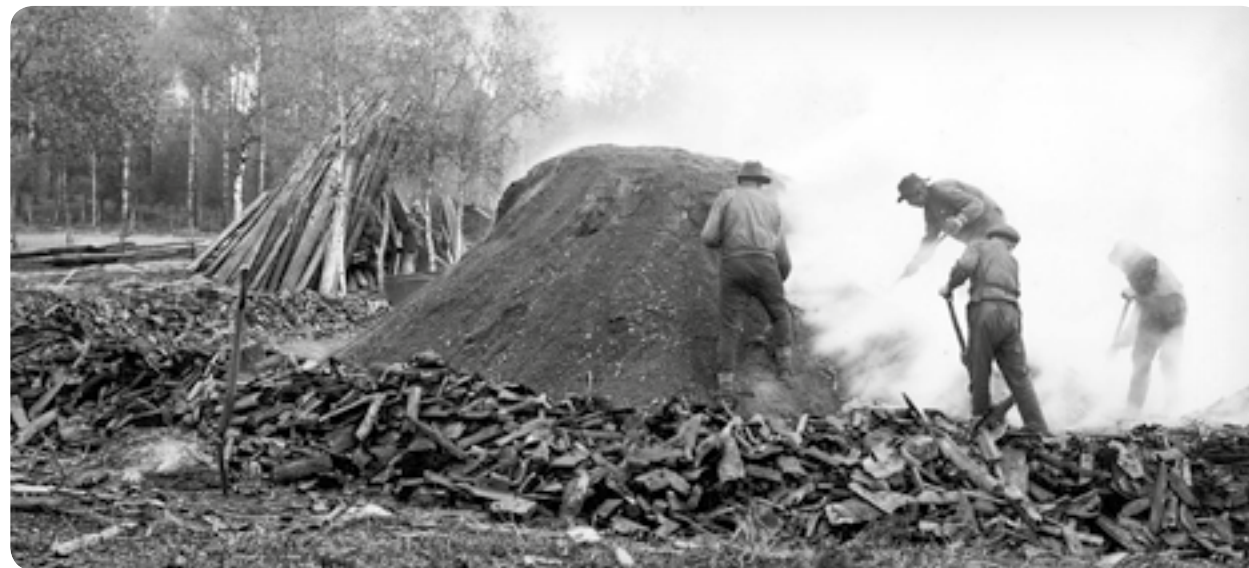
The need for charcoal for iron production had an early, large-scale industrial impact on the forest. Sites with traces of charcoal production are commonly found throughout large parts of the country today.
