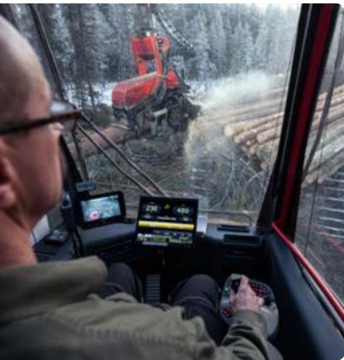
The machine in the picture, the harwarder, is a machine that both harvests and transports the timber. This is a Holmen-driven project that is intended to reduce both operating costs and environmental impact. Anders Lidén, Norsjö, Västerbotten.
