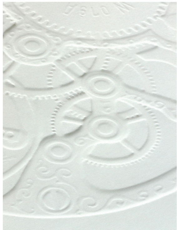
Embossing and debossing may be carried out either "blind" or combined with other techniques.
