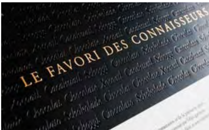
Hotfoil stamped, printed with four colours, varnished and finally embossed.
