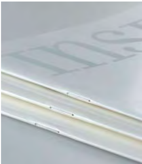
Saddle stitching puts a lot of strain on that small piece of paperboard that holds the cover to the insert by the staple.
