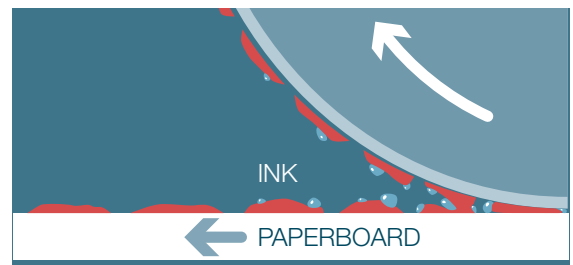
Fountain solution that is either non-emulsified or non-absorbed may obstruct ink transfer to both printed and unprinted surfaces.
